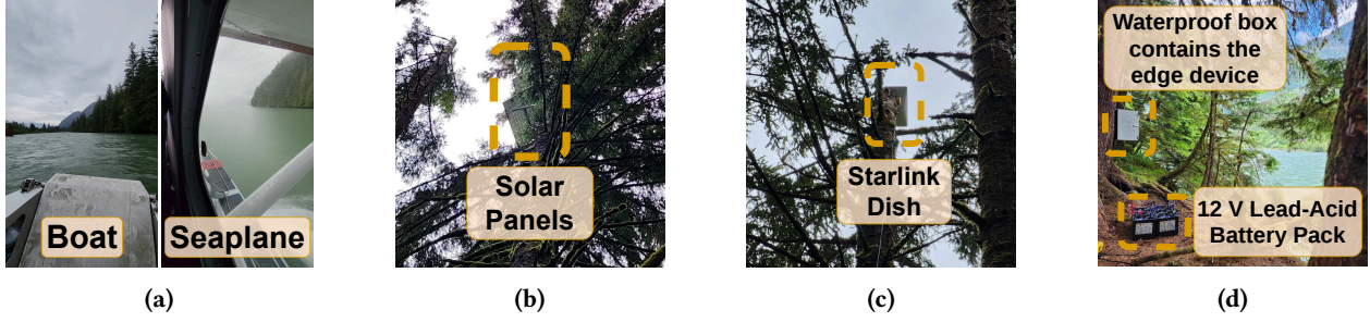
Figure 1. (a) Reaching deployment sites often requires multiple modes of transportation, including boats and seaplanes, making site visits costly. (b, c) A typical remote wildlife monitoring deployment in a temperate rainforest, with solar panels and the Starlink user terminal (UT) mounted in the tree canopy to maximize sunlight exposure and minimize signal obstruction, respectively. (d) Edge system hardware, including the edge computing enclosure and battery pack.
